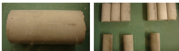
图7 浸水 32 d 后的淤泥固化土试样 Fig.7 Solidified sediment samples suffered from 32 d water immersion
